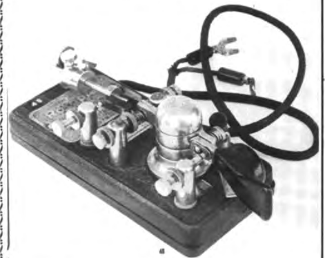
● (48) ROTOPLEX. U.S. Signal Corps Mfr. H.G. Martin Co. (1943) For use with Xmtr M.S. 738 (Clark Co. Louisville KY)
